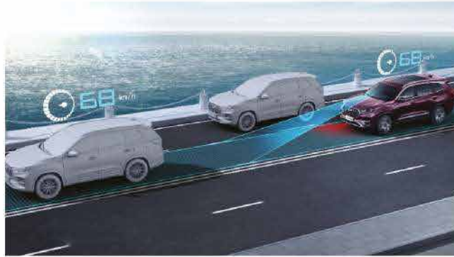
Autonomous Emergency Braking
